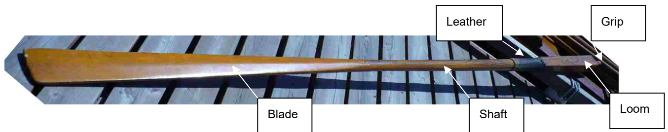
Figure 7-3. Parts of an oar
